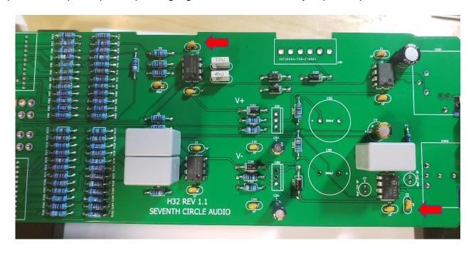
7. Install U1, U2, U3 and U4 now. Pay close attention to the IC markings. Align the notch on the IC with the notch on the silkscreen outline! IC sockets are not included in the kit and are not recommended. Socketing the ICs will interfere with the ability of the PC board to conduct heat away from the parts.
