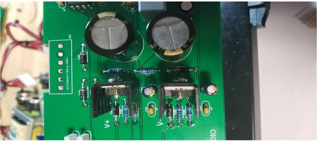
**16.** Before going on to initial power-up, carefully check your work. Make sure you haven't created any solder bridges between pads, or between a pad and the ground plane.
