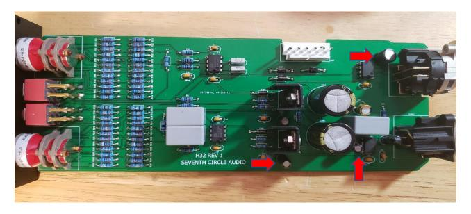
**10.** Carefully mount the toggle switches SW101 and SW201. Be sure they're seated flat on the board before soldering all the pins. You may find it easier to solder the first pin with the board component side up.
