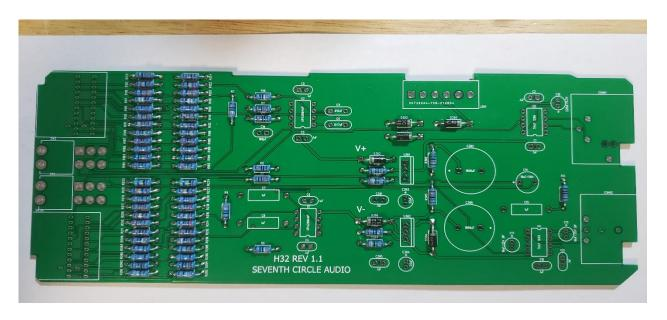
5. Next, add the protection diodes. Diodes are polarized and must be installed the right way around! The colored band on the diode matches the white band on the silkscreen.
