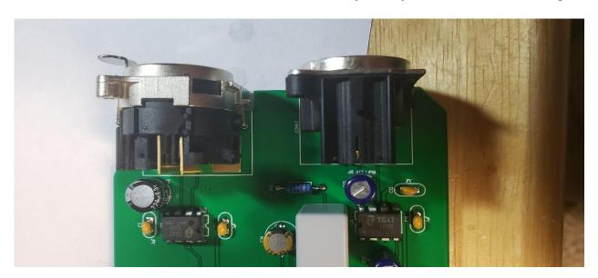
15. Install the bulk filter capacitors C302 and C305. Push them in firmly until they are fully seated against the board. Again, electrolytic capacitors are polarized and must be installed the right way around! Be absolutely sure to observe the correct polarity when installing these parts.
