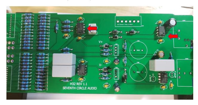
**8.** Install the 1uF film caps at C7, C8 and C15. These parts are not polarized and can be installed in either direction.
