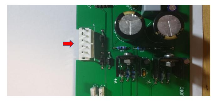
**12.** Using the hardware supplied, attach heat sinks to U301 and U302 and solder them in place. **Make sure to install the regulators correctly!** These parts are not the same and are not interchangeable.
