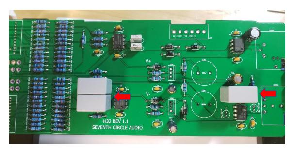
9. Add the electrolytic capacitors now. C13 and C17 are not polarized, but the rest are and must be installed the right way around! Be absolutely sure to observe the correct polarity when installing these parts. The negative leads of the electrolytic caps are marked with a colored stripe. The positive pads on the circuit board are marked with a small "+" sign.
