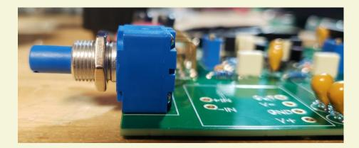
**17.** If it hasn't been already, insert the stop pin in rotary switch SW1 at the position shown. Push the pin in completely.
