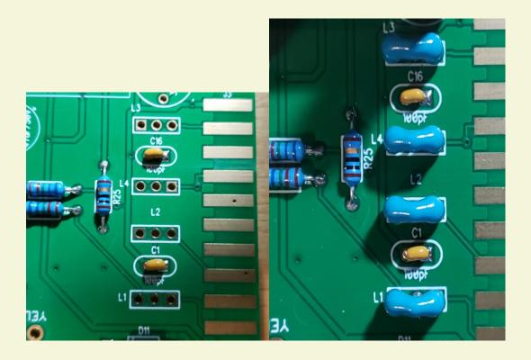
7. Add film capacitors. These capacitors are not polarized and can be installed in either direction. They may be a different color and/or shape than in the picture.
