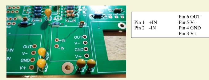
**25.** Again, carefully check your work. Make sure you've got the right resistors in the right locations. Make absolutely sure you've got all the diodes and capacitors soldered in the right way around! Double check to make sure you haven't inadvertently swapped a voltage regulator. Check for poor solder joints and solder bridges, and make sure you fix any problems before continuing.
